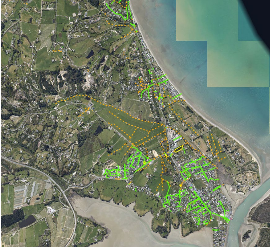
Figure 0-8: Māpua Ruby Bay Stormwater pipe and open channel network
