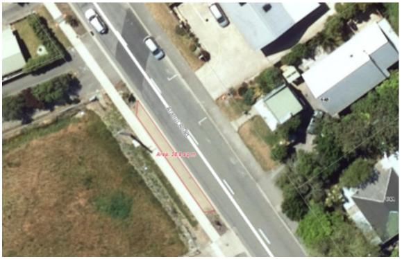
2. Removal of the low timber fence along the front of the reserve at the north end of Aranui Road, this will allow topsoiling and seeding of the batter between the new path and the reserve.
