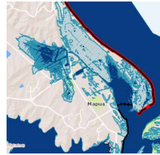
3. Salt-water intrusion under 0.5M sea-level rise, mean spring high tide mark (solid blue) and 1% annual exceedance probability (hatched blue)
