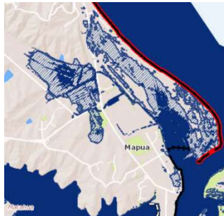
2. Current high tide mark (solid dark blue) in spring and 1% annual exceedance probability for salt-water intrusion (hatched dark blue)
