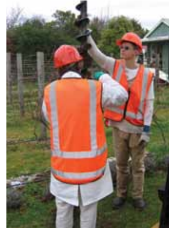
Soil sampling with an auger at Mapua during remediation
